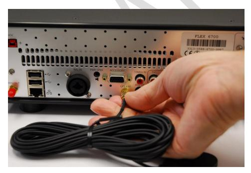
Using the double-sided adhesive oval that was included with the patch antenna, mount the GPS patch antenna on a window with a good view of the horizon.
