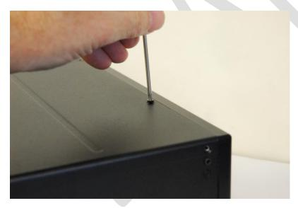
Using the long portion of the "L" TORX wrench install the three (3) short **Bottom Cover Side screws** on the **left** side of the FLEX-6000. Then install the remaining three (3) short Bottom Cover Side screws on the **right** side of the FLEX-6000. The image below shows the installation of the left side bottom Cover Side screws
