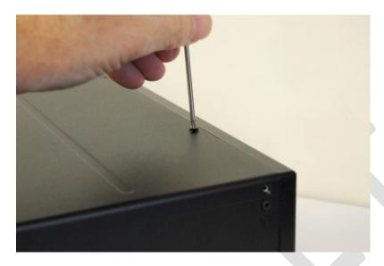
Once the bottom cover retaining screws have been removed, gently pull the Bottom Cover upwards to remove it from the FLEX-6000. The image below shows the removal of the Bottom Cover.
