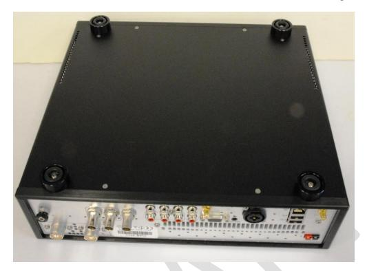
Turn the FLEX-6000 over and place it on its feet. The FLEX-6000 back panel should look like the image shown below with the two (2) gold SMA connectors for the GPSDO module installed.
