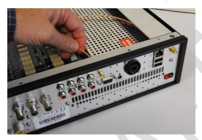
While firmly holding the cable assembly in place with one hand, insert the lock washer on the threaded SMA connector. Carefully install the SMA connector 5/16" (8 mm) hex nut on the threaded SMA connector being careful not to cross thread the SMA connector. Tighten hex nut with your fingers so that the coax cable assembly will freely rotate.
