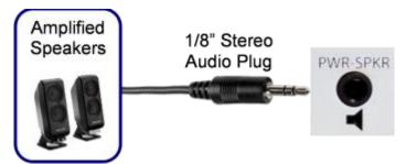
The powered speaker connector is a 1/8" TRS stereo connector. Stereo powered computer speakers should be used with this connector. Tip is the left channel, Ring is the right channel and Sleeve is common. The audio level is a nominal standard consumer (-10 dBV) line level. Do not use a mono or TS connector that grounds the "ring" portion of the connector.
