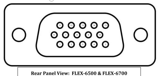
The accessory connector is a high-density HD-15 female connector. (This is the same connector used by VGA monitors.) There are a number of inputs and outputs on this connector.
