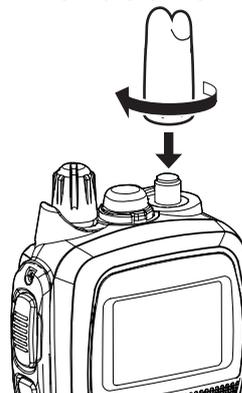
Connect the supplied flexible antenna to the antenna connector.
