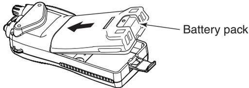
② Lock the battery pack with the latch.
