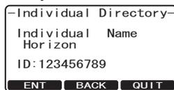
If a mistake was made entering in the MMSI number repeat pressing the **BACK** soft key until the wrong number is selected, then rotate the **CH** knob to correct the entry.
