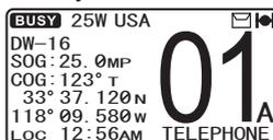
4. To stop dual watch, press one of the soft keys, then press the **DW** soft key again.
